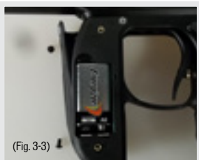
Note: Some rechargeable batteries are too large for the MINI GS battery compartment. If they don't fit, please don't force them as this may damage the board.
